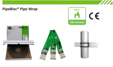
PipeBloc<sup>®</sup>Pipe Wrap is designed and tested to seal service penetrations in apertures containing combustible plastic pipes and pipes with insulation. The expanding wrap fills the void left by combusting materials and remains in place, exerting a pressure on the surrounding substrate upholding the fire resistance of the compartment. These are available in set size wraps (PipeBloc PWP Wrap) or in a 25mtr roll (PipeBloc EL).
