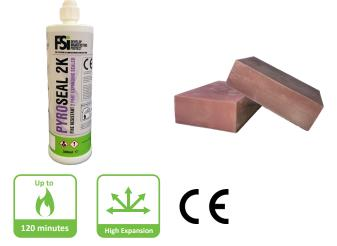
**PyroSeal 2K Expanding Sealer** is a 2-component polyurethane sealant system, manufactured with halogen-free intumescent fire retardants. On application the two components are mixed through a screw nozzle resulting in a reaction which causes the product to expand and swell around penetrating services.
