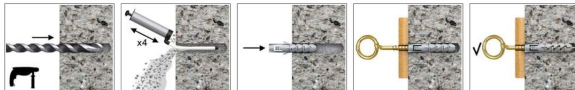
1. Drill a hole of required diameter.
