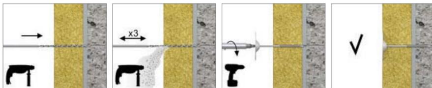
1. Drill a 5mm diameter hole perpendicular to the surface of the substrate
