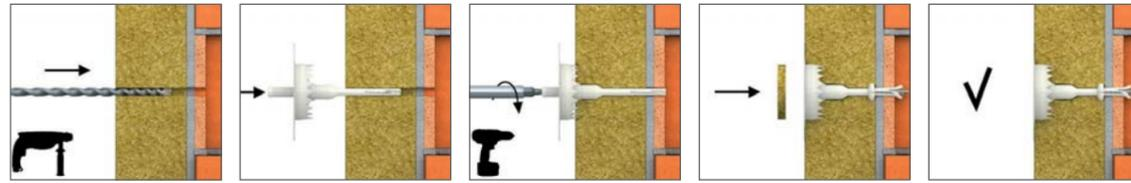
1. Drill a hole of required diameter and depth
