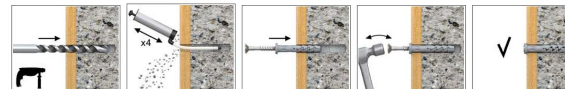
1. Drill a hole of required diameter.
