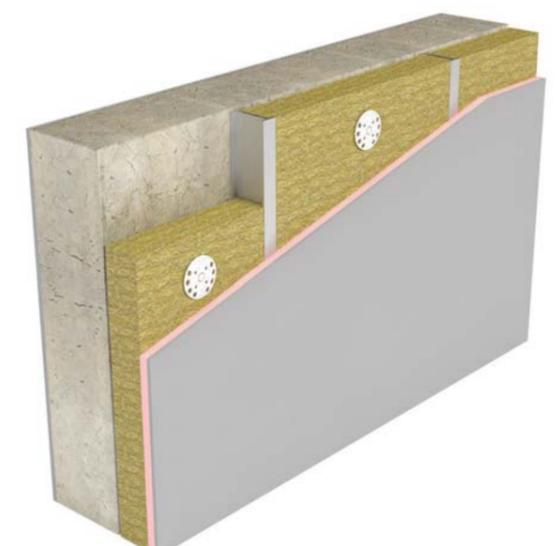
For each of the insulation methods we recommend a professional system of mechanical connectors, which serves as the fixing of the system to the elevation.
