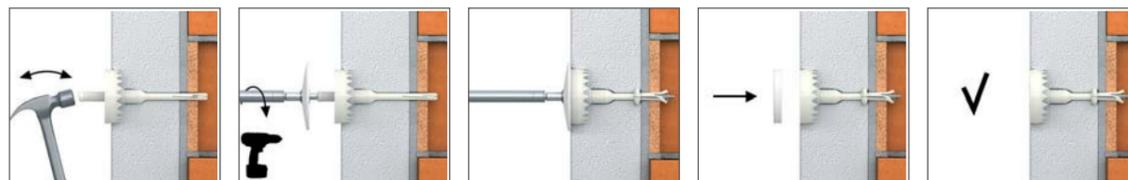
1. Drill a hole of required diameter and depth
