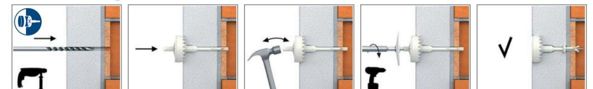
1. Drill a hole of required diameter and depth
