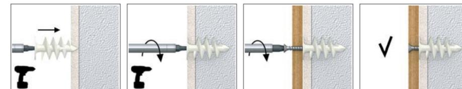
1. Drive ISO-PLUG into the insulation material (manually, or with an electric screwdriver) until installation depth reached.
