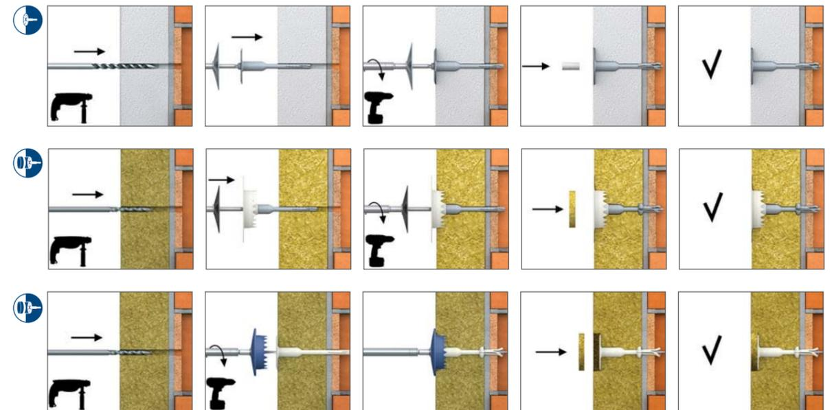
1. Drill a hole of required diameter and depth.
