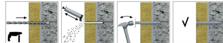
1. Drill a hole of required diameter and depth
