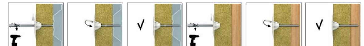
1. Lightly insert KC washer into surface of insulation material.
