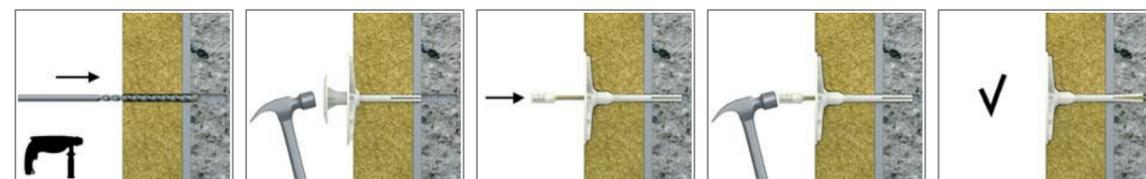
1. Insert chosen TFIX or KI fixing through hole in centre of KWL flange.
