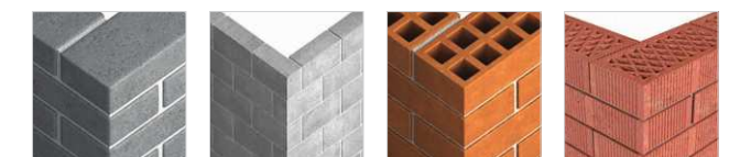
solid brick (ceramic or silica) lightweight concrete hollow brick hollow block
