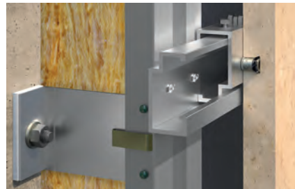
Façade cross-section with flush installation
