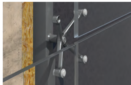
Façade cross-section with single layered glass panel
