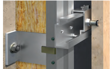
Façade cross-section with stand-off installation
