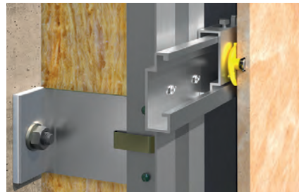
Façade cross-section with ceramic anchor
