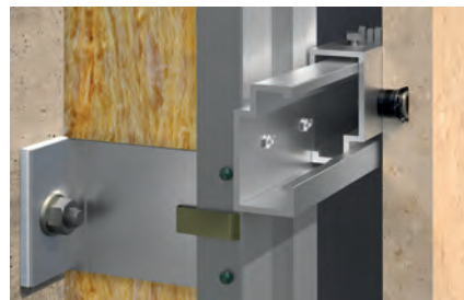
Façade cross-section with internal threaded anchor
